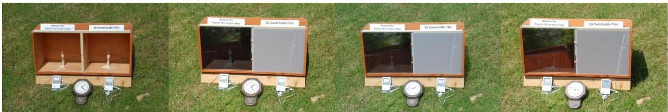
This experiment uses two isolated and sealed thermal chambers covered with a window film on glass and 3G Film on glass separately. The result shows that both temperature raising speed and the highest temperature in 3G Film chamber (right) are same as those in left chamber covered with popular window film sold in Home Depot with claim 70% of sun heat rejection.
